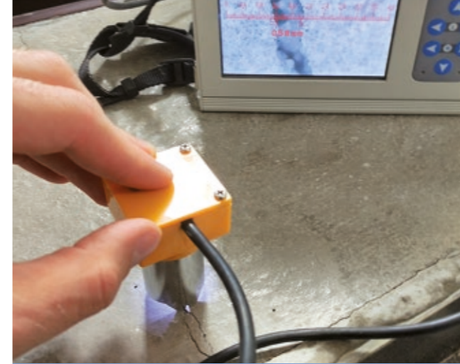
Above: Measuring plastic shrinkage cracks by digital microscope Below: Pressure layer built with DURUS EasyFinish concrete reinforcement
