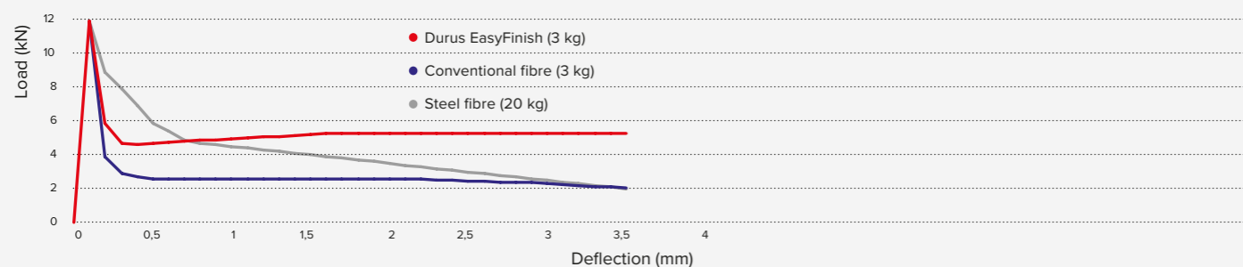
Fig. 4 / Three-point flexural bending test according to EN 14651
